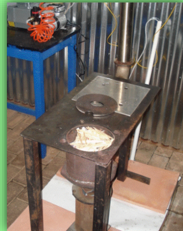
Mark IV 5 kW experimental downdraft stove
