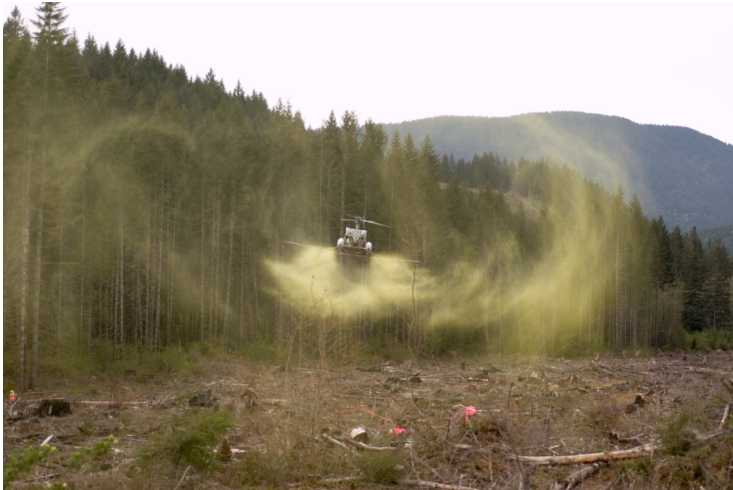
Figure 1. A Bell 47G3-B2A spraying a yellow fluorescent dye in water at a rate of 46.8 \text{ L ha}^{-1} with a fine (VMD of 126 \mu\text{m} ) droplet size distribution. Note the definite vortices generated at the rotor tips as delineated by the dyed spray (Thistle et al. (2009), photograph by Jim Kautz, USDA Forest Service).
