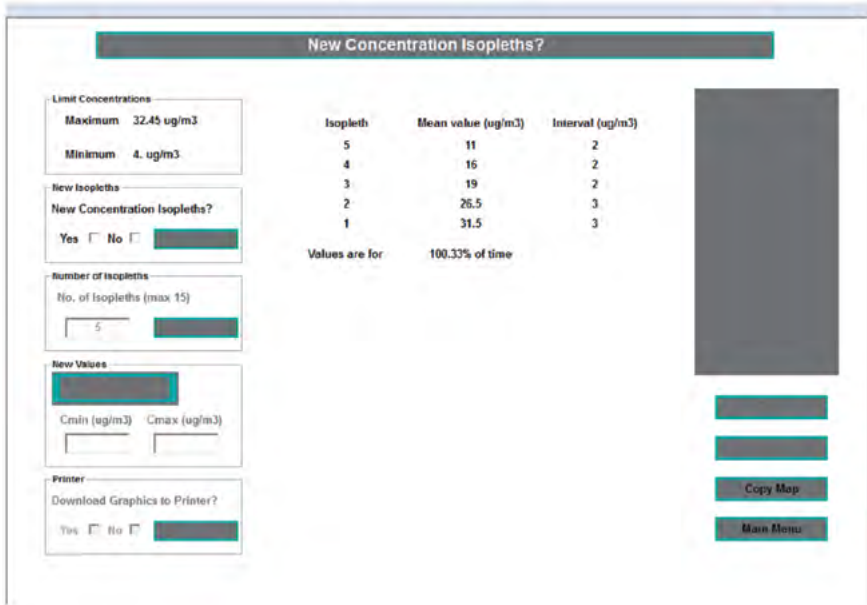
Figure 12 – Choosing isopleths for Spring 1982 with Holland plume rise and Pasquill dispersion – 196m altitude receptor (chosen by the user).
