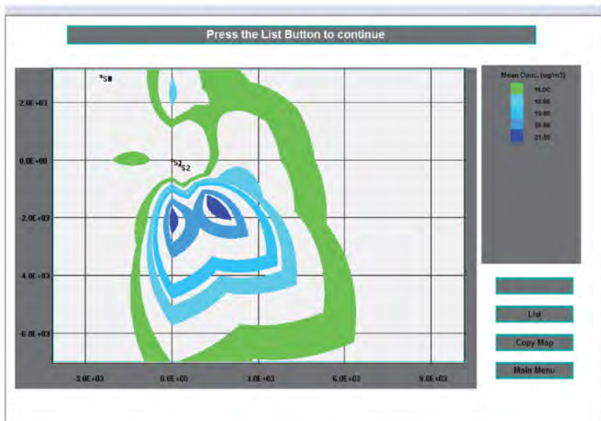
Figure 13 – Isoleths for Spring 1982 with Holland plume rise and Pasquill dispersion – 196m altitude receptor (chosen by the user as per Figure 12).
