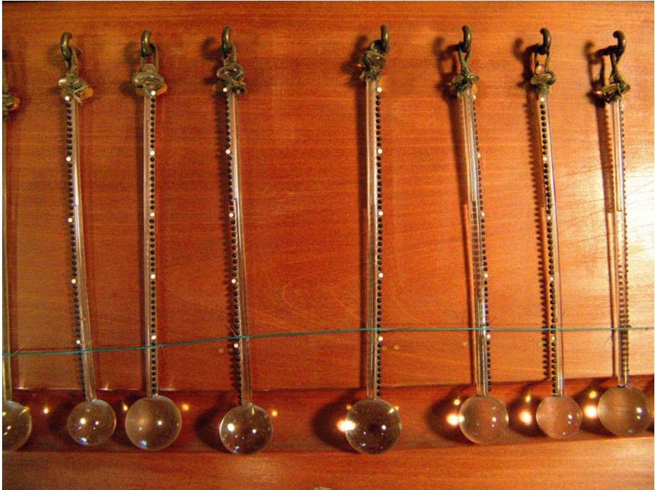
Fig. 2 Little Florentine Thermometers with 50°C scale marked with black and white glass enamel beads sealed on the glass tube. By courtesy of MG-IMHS, Florence
