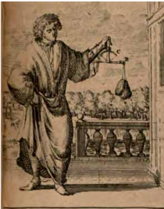
Fig. 1 Absorption hygrometer: a balance was used to detect changes in weight of a hygroscopic sample (D'Alancé 1707)
