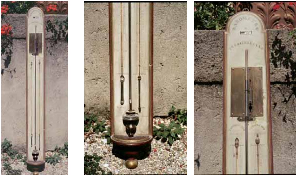
Fig.11 Original Chiminello's weather station kept at the Botanical Garden of the Padua University, composed of Réaumur thermometer, Torricelli cistern barometer and goose quill hygrometer. Details of the bulbs and the top of the tubes. Please note that the bulb thermometer and the quill have almost the same volume, and that the capillaries of these two instruments are identical and located side by side to make the temperature correction easier.
