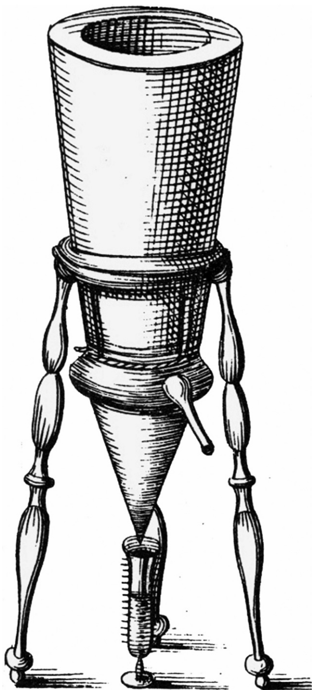
FIG. 18.7 Condensation hygrometer by the Grand Duke of Tuscany, Ferdinand II, and Evangelista Torricelli. The brass cone was filled of ice and the condensed water was collected on the graduated vessel under the cone. The cone has an exhaust pipe to drain melted water. From Magalotti (1667).
