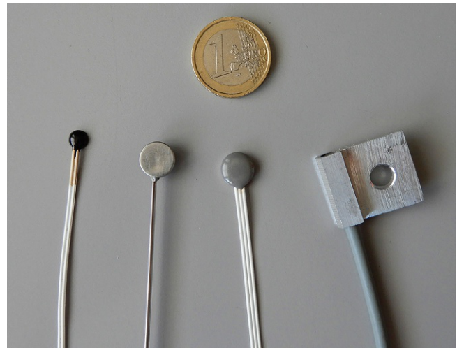
FIG. 17.21 Contact sensors and 1 Euro coin for size reference. The first and the third are viewed from the epoxy insulation on the top; the second from the stainless steel contact surface; the fourth has a hole to be fixed with a screw. Screws may be convenient for common use, hardly for cultural heritage.
