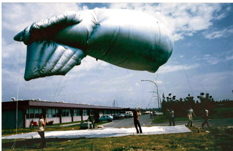
FIG. 17.18 A tethered kytoon used as radiosonde carrier. The kytoon is shaped like a traditional aerostat but with floppy wings at the back. In the case of wind, air blows into the wings through some inflation holes; wings are self-blown up and the kytoon becomes stabilized. Launching from the CNR campus, Padua, in the late 1970s.
