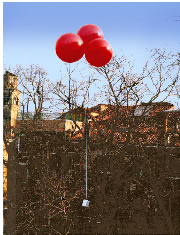
FIG. 17.19 A mini radiosonde (white box) carried by a cluster of three small weather balloons, launched from the Papadopoli Palace garden, in Venice. The white line connecting the radiosonde to the balloons is the transmitting antenna.
