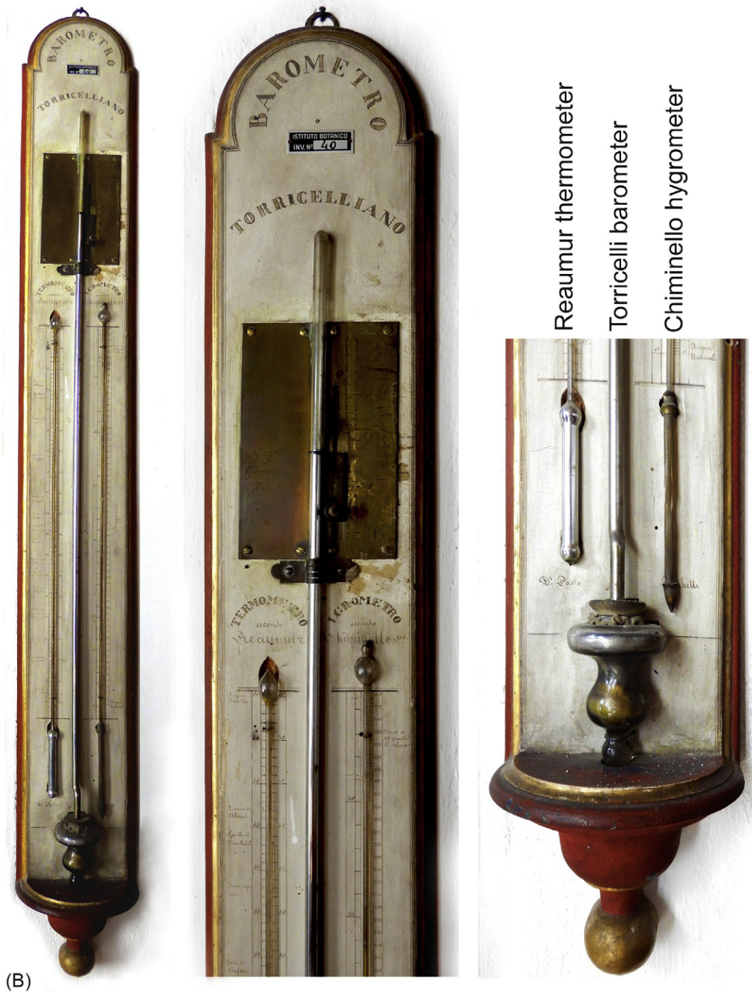
FIG. 18.6—cont'd (B) General view and details of the upper and lower ends of an early 'weather station' composed by Réaumur thermometer, Torricelli barometer, and Chiminello goose quill hygrometer. (A) From De Luc (1773–74); (B) Courtesy of the Library of the Botanical Garden, University of Padua, © Used with permission.
