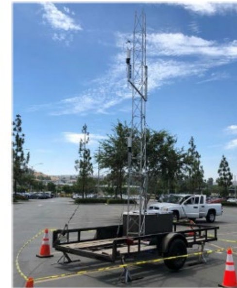
Fig. 4 Upwind meteorological measurement site containing two 3-D sonic anemometers mounted 3 m and 5 m above the ground
