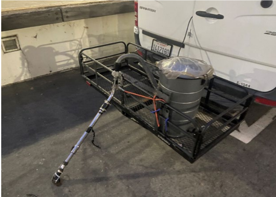
Spring-loaded arm keeps brush on the road
