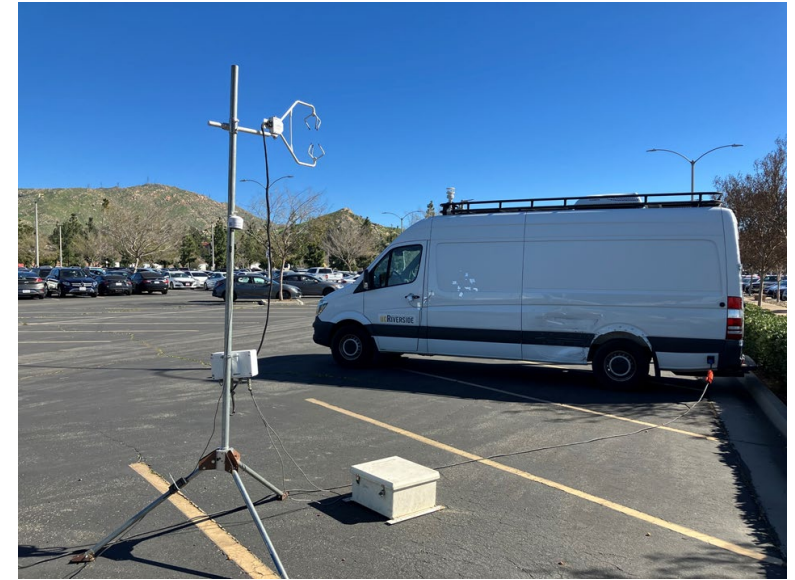
Measurement of micrometeorology using mobile monitor
