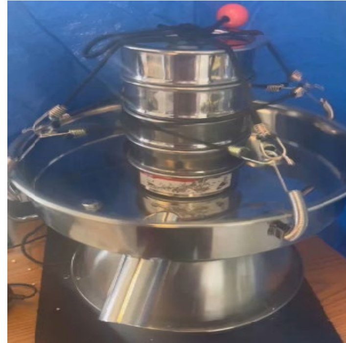
Silt collected using sequential sieving machine
